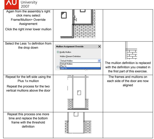
The right click menu of a curtain wall, unit or door/window assembly allows you to directly override definitions of these objects in the drawing. You could complete this exercise using only the Right click override functions:
